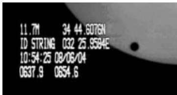
Fig. 1 – STVASTRO four-line output example: Elevation, Latitude, ID STRING, Longitude, Time (hh:mm:ss), Date (dd/mm/ yy) and Frame Field times (xxxx.x msec)
