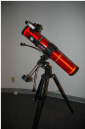
4.5" Tasco reflector with a manual German equatorial mount & tripod. Red and Black. $125.00
