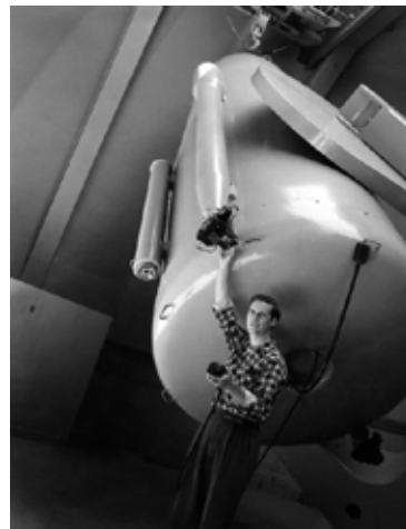
The Palomar Survey 48-inch survey telescope
