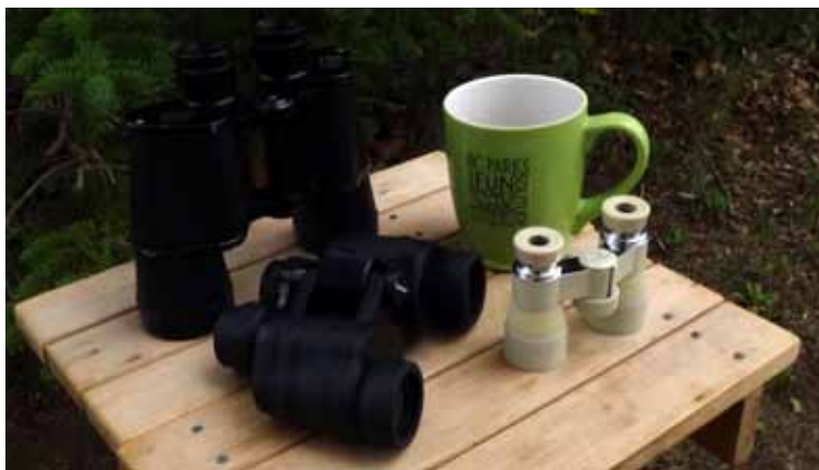
10 by 50 mm binos (standing), 7 by 35 mm wide field binos, (reclining) and 4 by 30 mm opera glasses (white)
