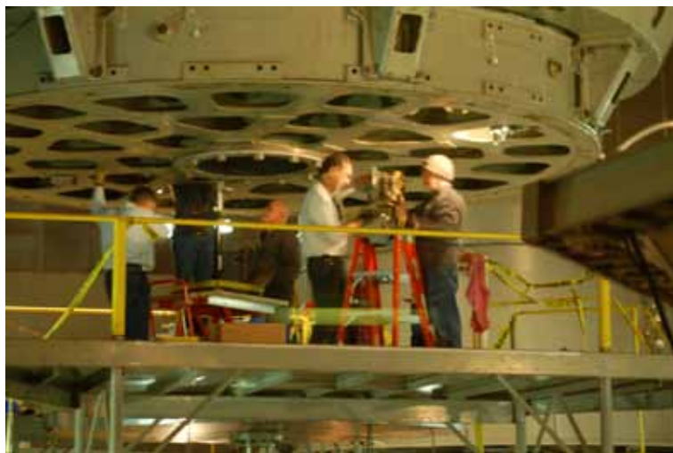
The Mirror Cell of the 200-inch Hale Telescope
